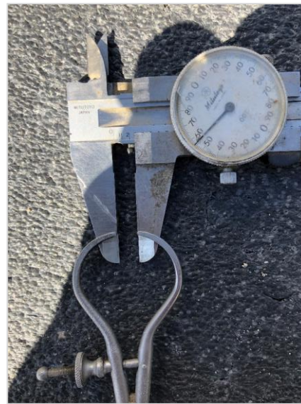
Photo 4. Flange Thickness Measurement
